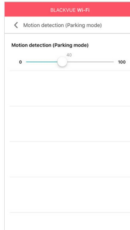
In parking mode the dashcam continuously buffers video and saves a parking recording when motion is detected in the dashcam's field of view.
