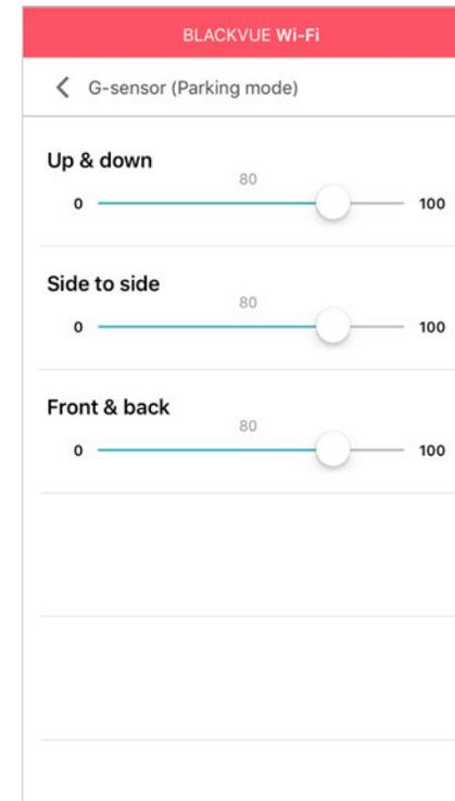
The G-sensor measures the movement of your vehicle through 3 axes – up and down, side to side, and front and back. When the G-sensor detects significant or sudden movement (such as an impact or collision) it will trigger an event recording. You can adjust the sensitivity so minor incidents and bumps don't trigger an event recording. To turn off event recordings by impact detection set the G-sensor sensitivity to zero.
