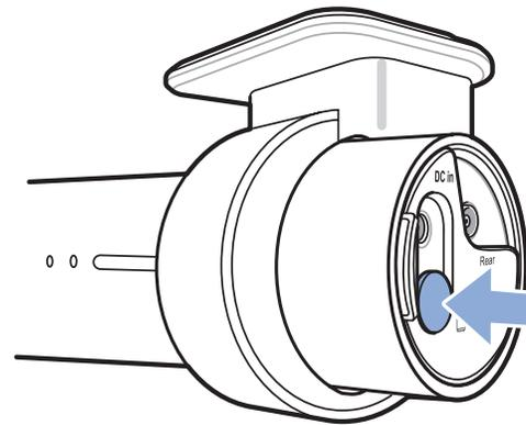
To format the microSD card press the Wi-Fi/Format button on the side of the dashcam for 10 seconds until the dashcam beeps.
